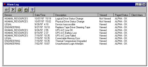
Figure 6 - The Alarm Log captures predicted and actual system faults.
