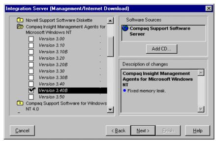
Figure 11 - Compaq Insight Manager shows the software resident on the Integration Server along with updates available from Compaq; you can download updates via the Internet, via a modem connection or from a local CD.
