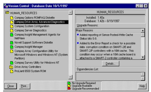
Figure 10 - Compaq Insight Manager shows the software resident on the Integration Server along with updates available from Compaq; you can download updates via the Internet, via a modem connection or from a local CD.
