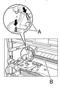
When removing the jammed paper, do not touch the transfer roller as its surface is very delicate and susceptible to finger oil and scratches, which may lead to print deterioration.
