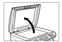
Clean the platen glass and the underside of the platen glass cover with a cloth dampened with water. Then, wipe the area with a soft, dry cloth.
