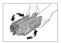
Insert the toner cartridge into the machine as far as it will go.
