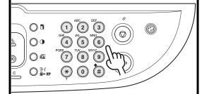
Enter the copy quantity (1 to 99) with the numeric key.
