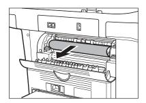
Carefully pull the jammed paper straight out through the rollers.
