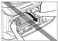
Do not pull the jammed paper upward.
