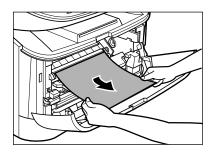
If the leading edge of the paper is visible but has not entered the imaging area, pull the paper forwards and roll it inwards.
