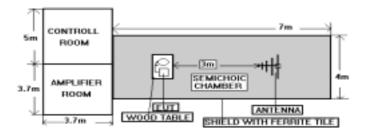
NOTE: The SPORTON 7m x 4m x 4m semichoic chamber is compliance with the sixteen points uniform field requirement as stated in IEC 1000-4-3 Section 6.2.
