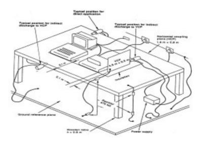
The test setup consists of the test generator, EUT and auxiliary instrumentation necessary to perform DIRECT and INDIRECT application of discharges to the EUT as applicable, in the follow manner:
