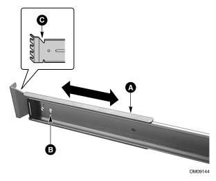
Figure 32. Attaching the Rail System to the Rear Rail Bracket
