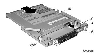
Figure 52. Removing a CD-ROM Drive from the CD-ROM Tray
