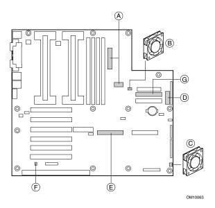
Figure 11. Connecting Cables to the Server Board
