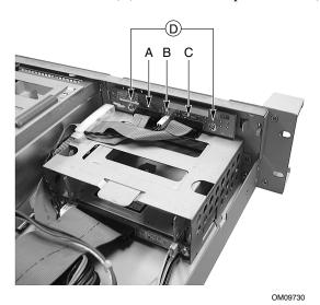
Figure 45. Replacing the Front Panel Board
