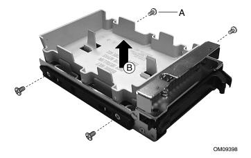
Figure 18. Removing the Air Baffles
