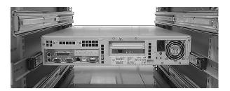
Figure 35. Chassis Mounted into the Rack
