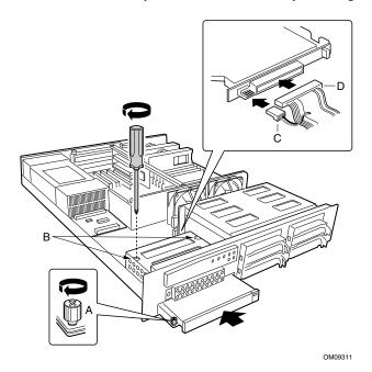
Figure 53. Installing a CD-ROM Drive
