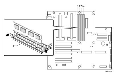
Figure 16. Installing Memory
