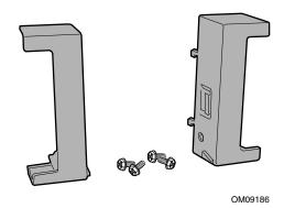
Figure 41. Bezel Mounting Hardware
