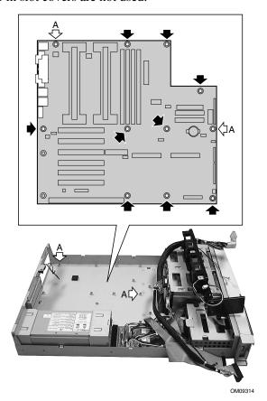
Figure 10. Mounting the Server Board on the Chassis Standoffs
