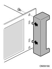
Figure 42. Attaching the Bezel Mount
