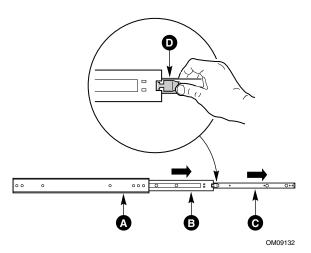
Figure 26. Chassis Rail System
