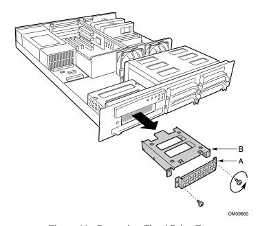
Figure 20. Removing Fixed Drive Tray
