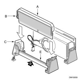
Figure 15. Installing a Termination Card
