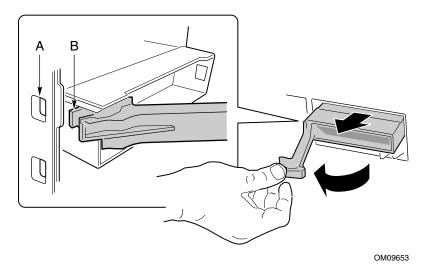
Figure 17. Removing the Hard Drive Carrier from the Chassis
