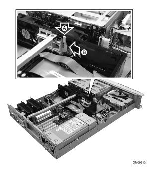
Figure 25. Using the Add-in Card Guide
