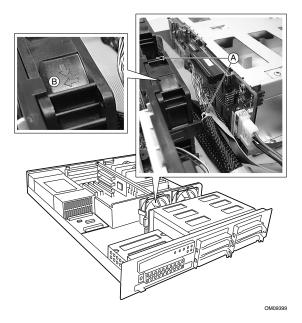
Figure 50. Replacing a Fan
