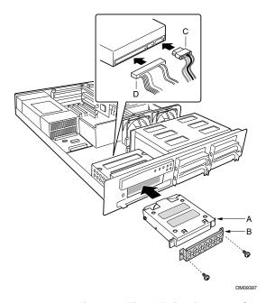
Figure 22. Installing the Fixed Drive into the Chassis
