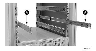
Figure 33. Extending the Rails
