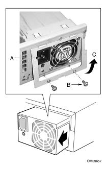
Figure 55. Replacing the Power Supply
