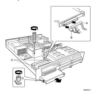
Figure 51. Removing the CD-ROM Drive
