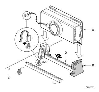
Figure 13. Installing a Primary Processor
