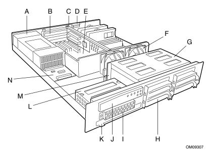
Figure 3. Major Internal Components of SR2000
