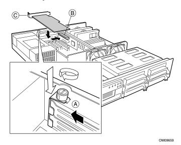
Figure 24. Installing an Add-In Card
