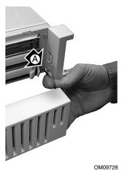
Figure 39. Removing Hinge Pegs from Bezel Mounts
