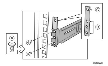
Figure 30. Attaching Rail Brackets to the Cabinet Rack
