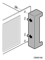
Figure 40. Removing the Bezel Mount
