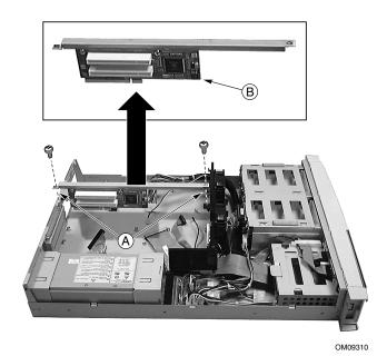
Figure 5. Removing the Riser Card
