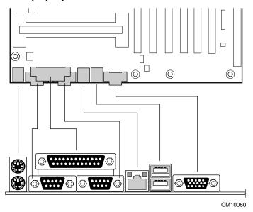
Figure 9. I/O Connector Edge of Server Board
