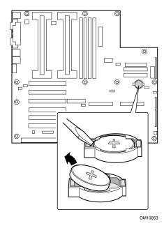
Figure 54. Replacing the Server Board Battery
