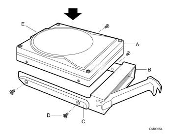
Figure 19. Attaching the Drive to the Carrier
