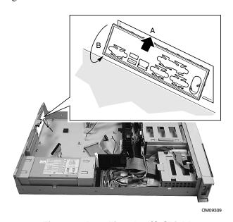
Figure 6. Installing the I/O Shield
