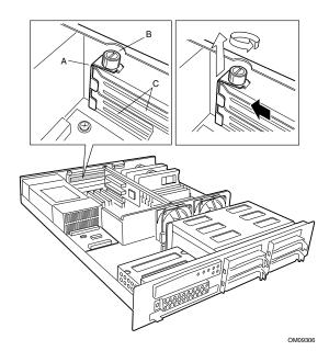
Figure 23. Removing the Slot Cover Retention Bracket
