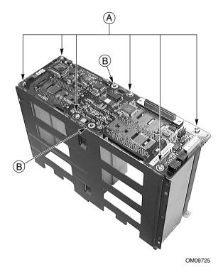
Figure 48. Removing the Hot Swap Backplane
