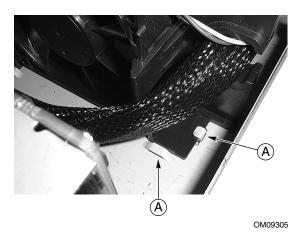
Figure 8. Removing the Fan Assembly from Chassis Tabs
