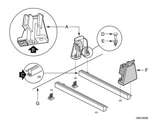
Figure 12. Inserting GRM Mounts for Processors
