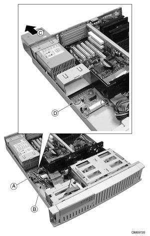
Figure 56. Removing the Power Supply Board
