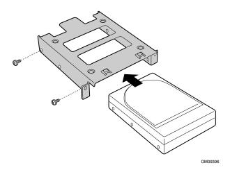
Figure 21. Installing a Drive into the Fixed Drive Tray
