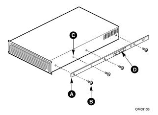
Figure 27. Aligning Rail to Chassis
