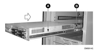
Figure 34. Guiding the Chassis into the Rack
