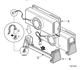
Figure 14. Installing a Secondary Processor
