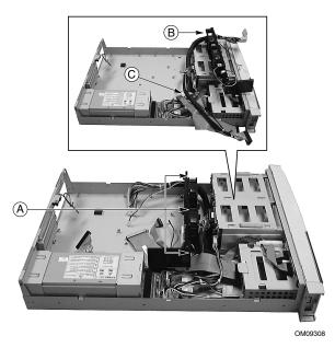
Figure 7. Removing the Fan Assembly Mounting Screws
