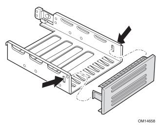
Figure 2. Removing the Plastic Cover
