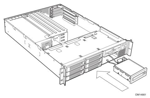
Figure 5. Installing the Tape Drive Assembly
