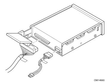
Figure 4. Connecting Cables to the Tape Drive
