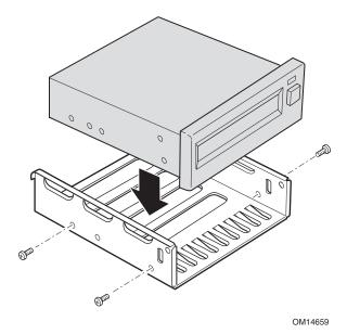
Figure 3. Installing the Tape Drive
