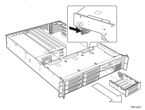
Figure 1. Removing the Tape Drive Carrier
