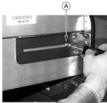
Figure 16. Chassis is Secured to Bracket with One Screw Noted by "A"
