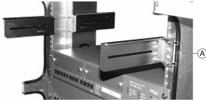
Figure 14. FR/RL Bracket Attached to the Rear Left Side of the Rack
