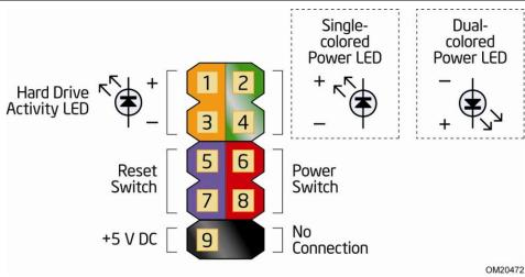
Figure 11. Connection Diagram for Front Panel Header
