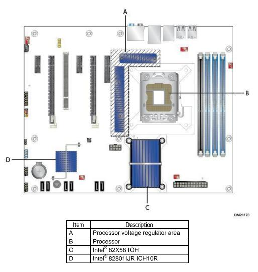
Figure 16. Localized High Temperature Zones
