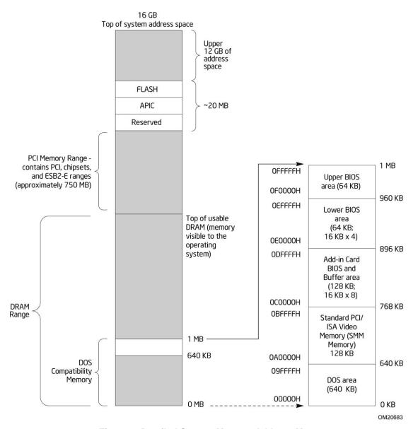
Figure 8. Detailed System Memory Address Map
