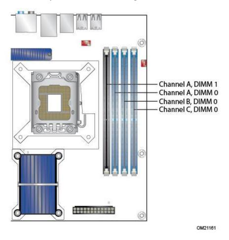
Figure 3. Memory Channel and DIMM Configuration
