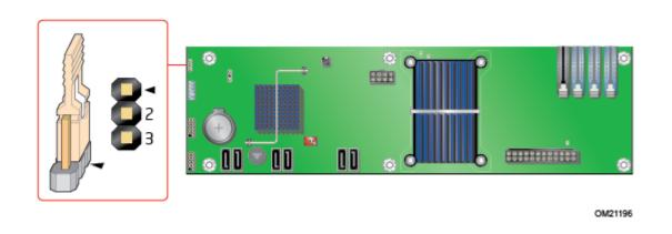
Figure 27. Location of the BIOS Configuration Jumper Block
