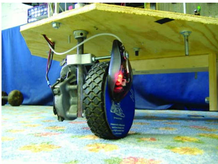
Figure 4. A Close-up of Our Optical Mouse Encoder
