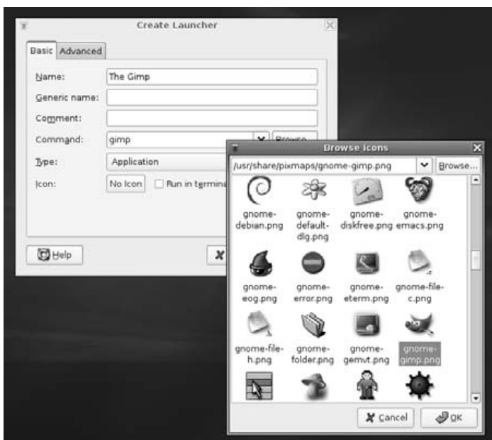
Figure 8. Creating a launcher is easy. Just fill in the Name and Command fields, and choose an icon.
