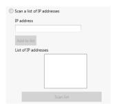
If a new device is found at an IP address provided, that device is added to the **New devices** group.
