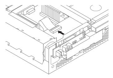
6. Remove the two screws holding the CD and diskette drive tray.
