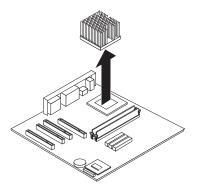
5. To remove the fansink from the processor, twist the fansink to break the seal formed by the thermal grease and remove.
