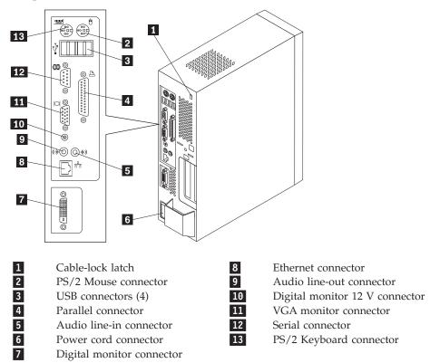
**Note:** Some connectors on the rear of your computer are color-coded to help determine where to connect the cables.
