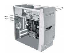
□ Slide the CD-ROM drive forward through the front opening and remove it.
