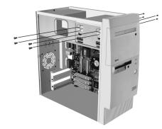
□ Slide the CD-ROM drive forward through the front opening and remove it.
