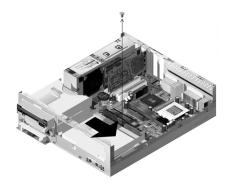
Pull the bay holder right to uncouple it from the chassis completely and lift it up.
