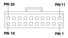
System Board Power Supply Connectors
