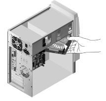
Remove the four screws (two on each side) that hold the diskette drive to the mounting tray
