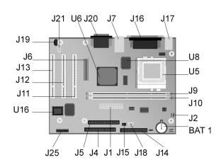
Layout of System Board of the Machine Type 2193 and 2196
