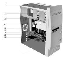
1. Power Supply This is a 95-watt switching power supply.
