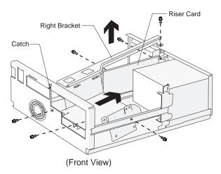
Figure 4-4. Right Drive Support Bracket
