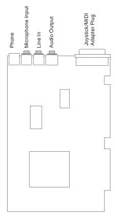
Figure 5-19. MWave Card (Combination Modem/Sound)
