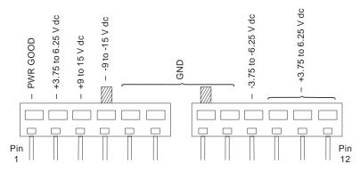
Figure 5-8. System Board Power Supply Connectors (J8 Bottom View)
