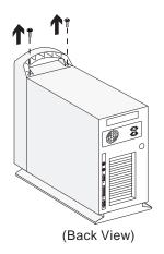
Figure 4-22. Remove the Screws
