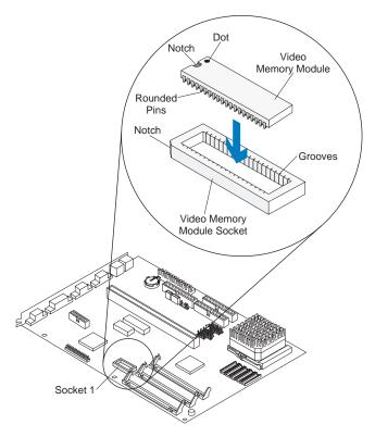
Figure 4-15. System Board Video Memory Module - Type H-1
