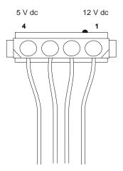
Figure 5-9. Hard Drive or CD-ROM End of Power Cable
