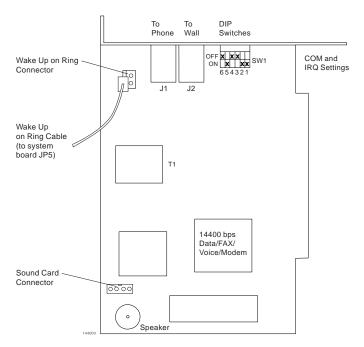
Figure 5-11. 14400 bps Data/FAX/Voice/Modem Card
