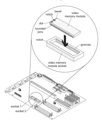
Figure 4-35. System Board Video Memory Module - Type H-2
