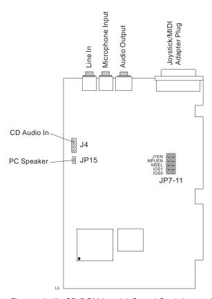
Figure 5-17. CD-ROM Level 3 Sound Card Jumper Settings
