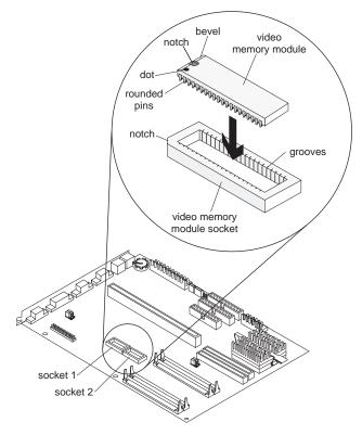
Figure 4-16. System Board Video Memory Module - Type H-2
