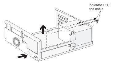
Figure 4-20. Indicator LED and Cable
