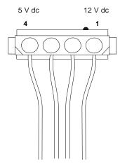
Figure 2-4. Hard Drive or CD-ROM End of Power Cable
