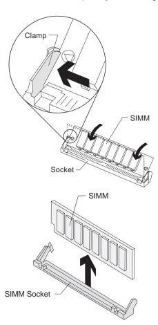
Figure 4-12. System Board SIMM Sockets
