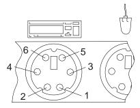
Figure 2-6. Keyboard Connector Voltage Check
