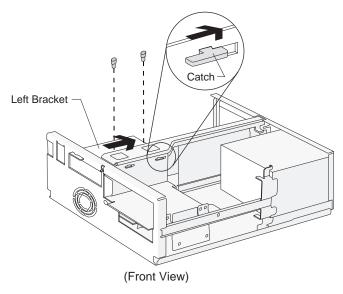
Figure 4-3. Left Drive Support Bracket
