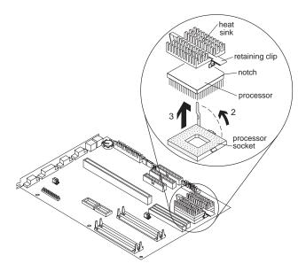
Figure 4-36. System Board - Type H-2
