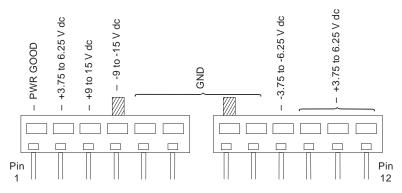
Figure 2-3. System Board Power Supply Connectors (J8 Bottom View)
