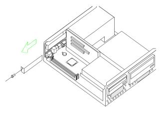
**2.** Align and insert the adapter card into the adapter card connector.
