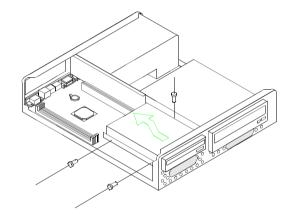
**3.** Slide the diskette drive backward from the front of the system unit and lift it up to remove it.
