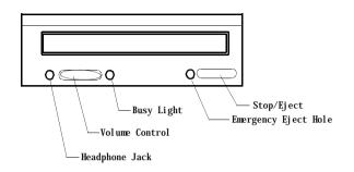
When your headphones are plugged into the headphone jack on the CD-ROM drive, they will pick up only the sound coming from an ordinary audio CD in the CD-ROM drive. The headphones will not pick up other sounds generated from your computer or any external device connected to the computer, such as a MIDI (Musical Instrument Digital Interface) keyboard.
