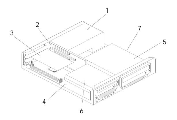
Your computer's system unit has 3 bays that can hold up to one 5.25-inch and two 3.5-inch drives.
