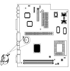
**3.** Insert a new 3V lithium battery (CR2032) into the socket and press it down until the securing clip clicks and locks the battery in.If you replace the system
