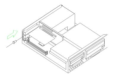
**4.** Reinstall all hardware (except for the slot cover, which cannot be reinstalled) and screws that you removed prior to the installation of the adapter card.
