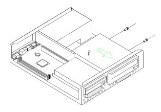
**3.** Slide the CD-ROM drive toward the front of the system unit to remove it.
