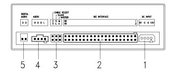
**NOTE:** CD-ROM drives may come with item no. 5 (digital audio output and testing jumper) connectors.
