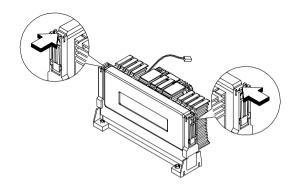
· Firmly hold the processor module and pull it out of the socket.
