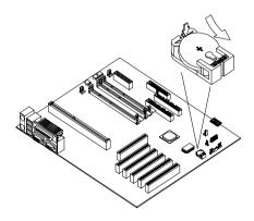
• If you replace the system battery, you need to reset the system date and time. You can perform this task from the Window 98 desktop or from the Setup Utility. To reset the system date and time in the Setup Utility, select the Date and Time option from the Main Menu.
