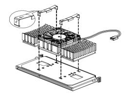
Press the fastener towards the fan sink side to lock the fan sink.
