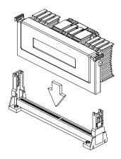
**CAUTION:** The electrical contacts of the AMD K-7 module are slotted in such a way that the module only fits in one direction. Make sure that the module groove matches the one on the processor socket.
