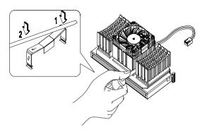
• To remove the fan sink, use a screw driver to slide the fastener nodes outward to unlock the fan sink from the processor, then carefully remove the fan sink from the processor.
