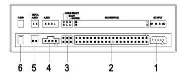
**NOTE:** CD-ROM R/W drives may come with item no. 5(digital audio output and testing jumper) connectors.
