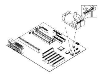
**IMPORTANT:** Make sure to insert the battery with the positive side facing up. A plus(+) sign indicates the positive side.
