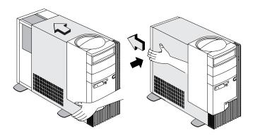
Turn the lock at the back of the system unit toward the "locked" icon to secure the cover to the chassis.
