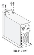
**b** Slide the cover forward and completely remove it from the system unit.
