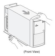
3 Touch the bare metal frame of your system unit to dissipate the static electricity from your body. Do not touch any of the components inside the frame before you touch the frame. Do not touch any component with a voltage warning label.
