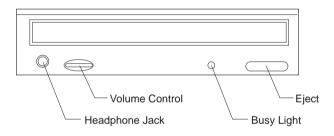
When your headphones are plugged into the headphone jack on the CD-ROM drive, they will pick up <u>only</u> the sound coming from an ordinary audio CD in the CD-ROM drive. The headphones will <u>not</u> pick up other sounds generated from your computer or any external device connected to the computer, such as a MIDI (Musical Instrument Digital Interface) keyboard.
