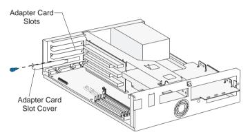
**2.** Align and insert the adapter card into the adapter card connector. Insert the screw.
