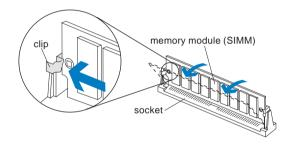
3. Lift the module out of the socket.
