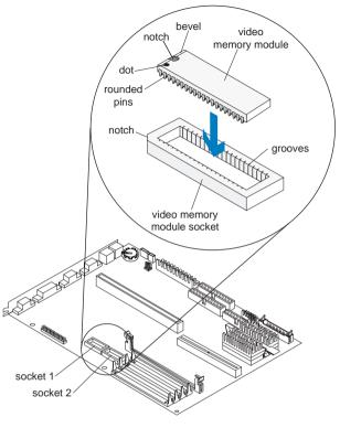
**3.** Align the rounded pins on the sides of the memory module with the grooves in the memory module socket.
