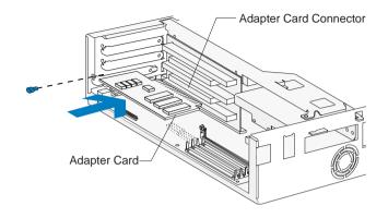
**3.** Reinstall all hardware and screws you removed to install the adapter card.
