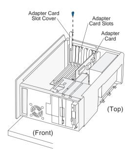
**3.** Align and insert the adapter card into the adapter card connector. Insert the screw.
