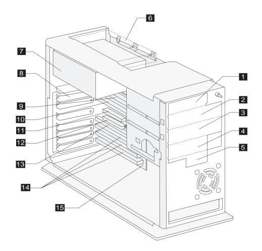
Your computer's system unit has six bays and can hold up to six drives. It also has seven adapter card slots and eight adapter card connectors and can hold up to seven adapter cards. You can purchase a drive to install in any empty bay or an adapter card to install in any empty slot.
