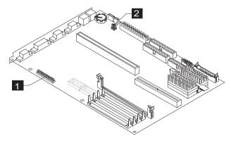
Note whether the location of the cable connector you need to use is beneath the riser card. If it is, follow the instructions in "If you need to remove the riser card in a minitower system" on page 64 before you install the new adapter card.
