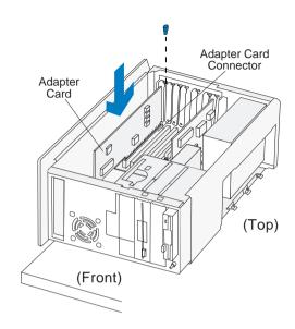
**4.** Reinstall all hardware and screws you removed to install the adapter card.
