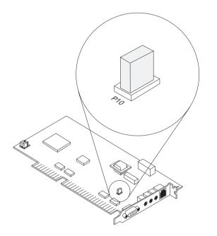
**2.** Move the jumper from the enabled position to the disabled position as shown in the picture.
