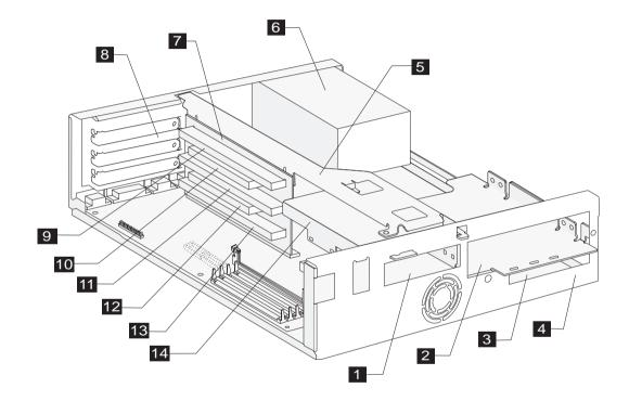
Your computer's system unit has four bays and can hold up to four drives. It also has three adapter card slots and five adapter card connectors and can hold up to three adapter cards. You can purchase a drive to install in any empty bay or an adapter card to install in any empty slot.
