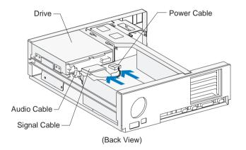
note: If you are adding a diskette or tape drive that attaches to the Diskette connector, make sure the signal cable you plug into the drive is attached to the Diskette connector on the system board. To identify the Diskette connector, see "Identifying signal cable connectors" on page 95.
