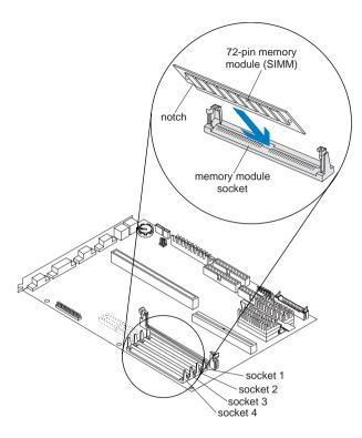
**3.** Press forward <u>firmly</u> on the memory module to move it into a vertical position. Both sides of the module will "click" when the module locks into place. The newly-installed memory module will be locked into the socket in a vertical position with pins showing through the holes on each side.
