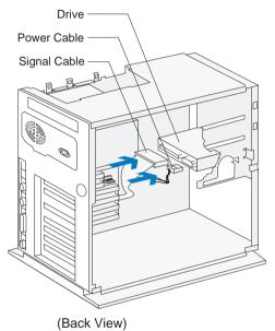
If you add a diskette drive or a tape drive that attaches to the Diskette connector, make sure the signal cable you plug into the drive is attached to the Diskette connector on the system board. To identify the Diskette connector on the system board, see "Identifying signal cable connectors" on page 118.
