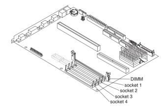
If your computer comes with 16MB installed on the system board, your DIMM and/or SIMM sockets are filled in one of the following configurations:
