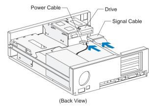
If you are adding a diskette or tape drive that attaches to the Diskette connector, make sure the signal cable you plug into the drive is attached to the Diskette connector on the system board. To identify the Diskette connector, see "Identifying signal cable connectors" on page 95.
