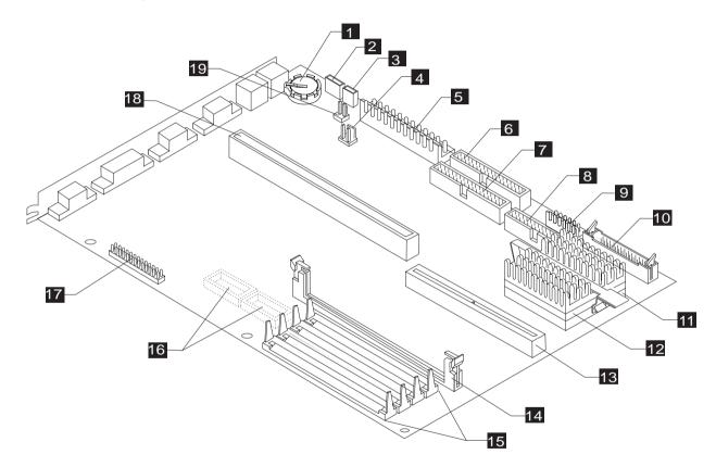
The *system board*, sometimes called the *planar* or *motherboard*, is the main circuit board in the system unit. It supports a variety of devices and provides other basic computer functions that are preinstalled or that you can install later. The system board shown on page 65 has the following parts:
