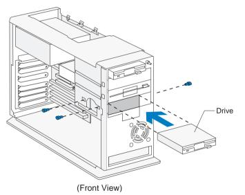
**2.** Connect the power and signal cables to the drive.
