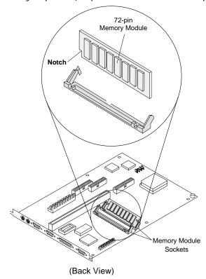
**3.** Press back *firmly* on the memory module until both sides *click*, locking into place. The newly installed memory module will be at an angle with pins showing through the holes on each side.
