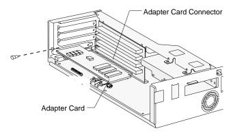
**4.** Plug your monitor cable into the video adapter card connector that extends from the adapter card slot out to the back of the system unit (instead of the monitor connector on the back of the system unit,
