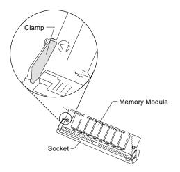
**3.** Lift the module straight out of the socket.
