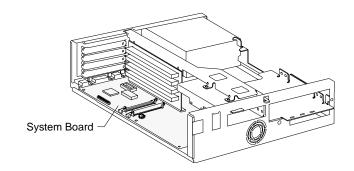
This is an example of how the system board is shown in "Working with your system board" in order to make the parts of the system board easier to see.
