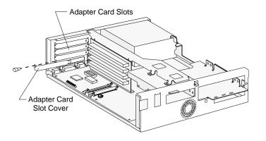
**b.** Align and insert the adapter card into the adapter card connector. Insert the screw. (Reverse this step for card removal.)
