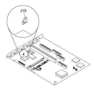
**2.** Lift the jumper from its current position (this could be Position 1 or Position 2). If the jumper is currently in Position 1, move it to Position 2. If the jumper is currently in Position 2, move it to Position 1. See the *example*.
