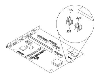
**2.** Lift the jumper from its current position (this could be Position 1 or Position 2). If the jumper is currently in Position 1, move it to Position 2. If the jumper is currently in Position 2, move it to Position 1. See the *example*.
