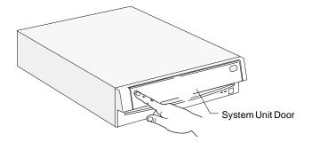
**b.** Press up on the release latch. Slide the cover off completely.
