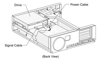
If you are adding a diskette, tape, or CD-ROM drive that attaches to the Diskette connector, make sure the signal cable you plug into the drive is attached to the Diskette connector on the system board. To identify the Diskette connector, see "Identifying parts of the system board" on page 92. If you are adding a CD-ROM drive, it is recommended that you use the ISA Bus connector on the system board.
