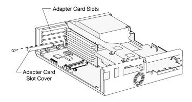
2. Align and insert the adapter card into the adapter card connector. Insert the screw. (Reverse this step for card removal.)
