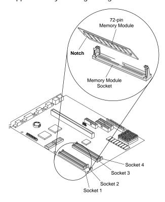
**3.** Press forward *firmly* on the memory module to move it into a vertical position. Both sides of the module will *click* when the module locks into place. The newly installed memory module will be locked into the socket in a vertical position with pins showing through the holes on each side.
