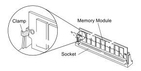
**3.** Lift the module out of the socket.
