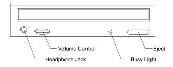
When your headphones are plugged into the headphone jack on the CD-ROM drive, they will pick up **only** the sound coming from an ordinary audio CD in the CD-ROM drive. The headphones will **not** pick up other sounds generated from your computer or any external device connected to the computer,
