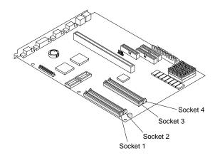
Socket 1 and Socket 2 work together as a set. Socket 3 and Socket 4 also work together as a set. When adding or replacing memory modules, you must fill both
