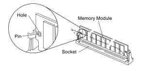
note: Remember to reinstall all hardware you removed to access the memory module sockets.
