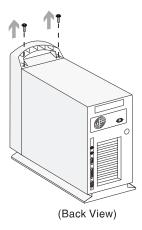
**b** Slide the cover forward and completely remove it from the system unit.
