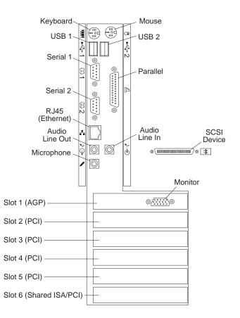
Note that the monitor connector is located on the graphics adapter installed in one of the expansion slots.
