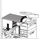
**3** Remove the two screws that secure the top and the bottom of the upper drive bracket, then disconnect the power and signal cables attached to the drives in the upper drive bracket.
