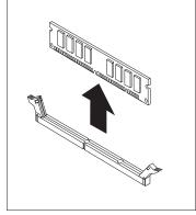
${f 6}$  Store the DIMM in a static-protective package.
