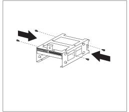
**5** Reinstall the lower drive bracket and secure it with the screw.
