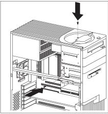
${f 6}$  Connect the power and signal cables to the drive(s).
