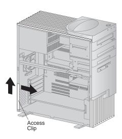
**3** Remove the screw and cover for the appropriate expansion slot.
