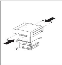
**5** Reinstall the upper drive bracket and secure it with screws at the top and bottom.
