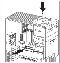
**6** Connect the power and signal cables to the drive(s).
