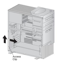
${f 3}$  Remove the screw and cover for the appropriate expansion slot.
