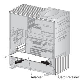
**4** Insert the adapter into a static-protective package.
