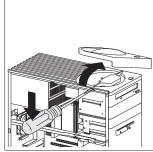
$\mathbf{3}$  Remove the two screws that secure the top and the bottom of the upper drive bracket, then disconnect the power and signal cables attached to the drives in the upper drive bracket.
