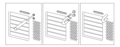
$oldsymbol{3}$  Replace the computer cover. For more information, see "Replacing the Cover and Connecting the Cables" on page 68.
