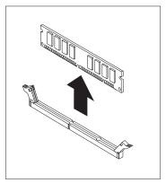
**4** Lift the DIMM out of the connector.
