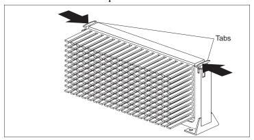
**4** Carefully place one hand on the computer frame and pull the microprocessor up and out of the connector with the other hand.
