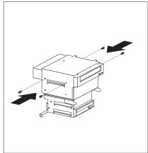
${f 5}$  Reinstall the upper drive bracket and secure it with screws at the top and bottom.
