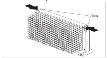
**7** Align the new microprocessor with the connector on the system board and slide it into the guides. Press the microprocessor down until it seats in the connector.
