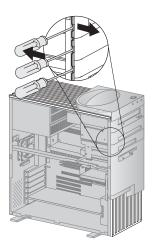
${f 2}$  Remove the top cover by using a flat-bladed screwdriver to release the tab on the left edge as shown.
