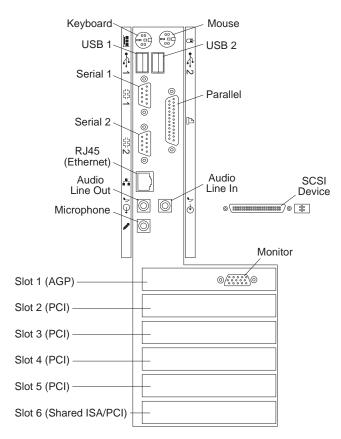
**Note:** The monitor connector might be in a different slot, depending on the computer model.
