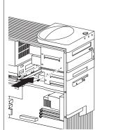
Attach the cables to the drives. If necessary, see page 80 for an illustration showing the locations of the drive connectors on the riser card.
