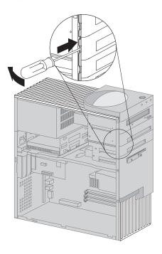
2. If knockouts are present in the drive bay opening, twist them with a screwdriver or pliers to remove.
