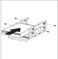
4. Reinstall the drive cage and secure it with the screw you removed in step 2.
