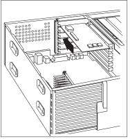
4. If you installed a network adapter that uses Wake on LAN or Alert on LAN, attach the cable from the riser card to the adapter. See page 80 to locate the Wake on LAN or Alert on LAN connectors.
