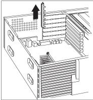
2. Remove the appropriate expansion slot cover.
