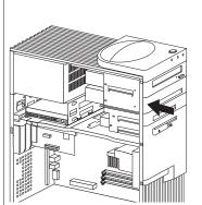
6. If you installed a CD-ROM drive and want to connect the drive to the CD-ROM audio connector, see page 80 to locate the CD-ROM audio connector on the riser card.
