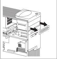
3. Install the drive in the bay opening and secure the drive by inserting screws.
