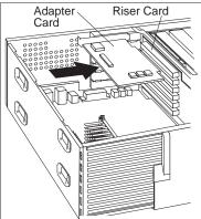
3. Install the bracket and the screw.
