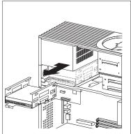
3. Slide the drive into the bay and secure it with rubber grommets and screws.
