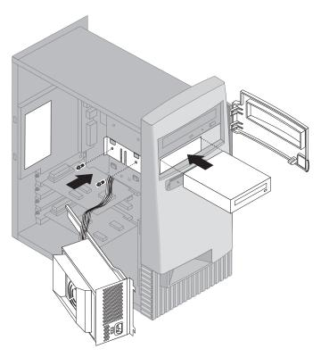
5. If the drive you installed has nonremovable media (such as a hard disk drive), replace the bay panel.
