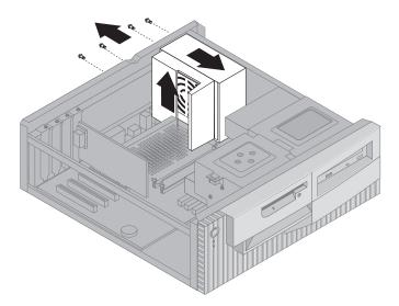
4. Rotate the power supply toward the system board slightly.
