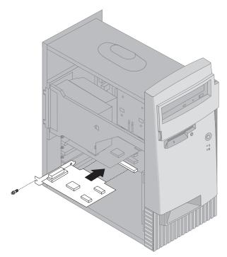
Note: If you are installing a Wake on LAN supported network adapter, attach the Wake on LAN cable that comes with the adapter to the Wake on LAN connector on the system board. (This might not be necessary with all computers.) If you also want to take advantage of the Alert on LAN feature of your computer, you must install your network adapter in PCI slot 3. For the location of PCI slot 3 and the Wake on LAN connector, see the diagram of the system board on the inside of your computer.
