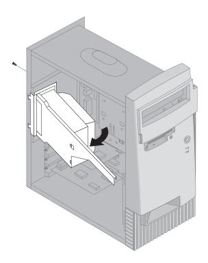
5. Pull the power supply forward and carefully rotate it toward the front of the chassis. Lay it to the side.
