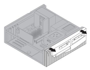
4. Insert a flat-blade screwdriver into one of the slots on the static shield in the drive bay into which you are installing the drive and gently pry the static shield loose from the drive bay.
