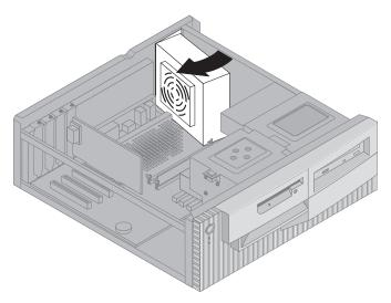
5. Lift the power supply up and carefully rotate it toward the front of the chassis. Lay it on the diskette drive bay, taking care to give yourself room to access the rear of the drive bay with which you are working.
