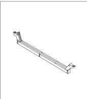
3. Make sure that the notches in the DIMM are properly aligned with the connector. Push the DIMM straight down into the connector until the retaining clips close.
