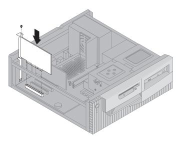
4. Install the screw that secures the adapter.
