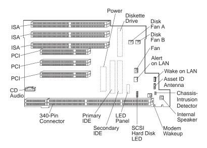
The riser card plugs into the system board via a 340-pin connector. Adapters plug into the ISA- or PCI-expansion connectors (slots) on the riser card. Signals from adapters are routed to the ISA or PCI buses. Each ISA-expansion connector provides a 16-bit-wide data path, and each PCI-expansion connector provides a 32-bit-wide data path.
