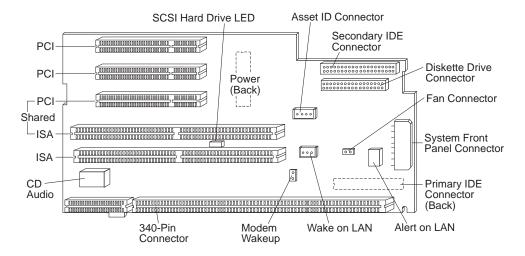
Each PCI-expansion connector is capable of driving one, low-power Schottky load. Each ISA-expansion connector is capable of driving two, low-power Schottky loads. The ISA bus is permanently set to the PCI bus speed divided by four.
