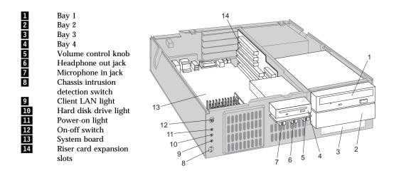
Your computer comes with a diskette drive installed in bay 4 and a hard disk drive installed in bay 3. If your computer comes with a CD-ROM drive, it is installed in bay 1; if your computer comes with a SCSI adapter, it is installed in an expansion slot.
