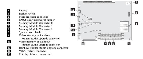
**Note:** An illustration of the system board and additional information are provided on a label found on the underside of the computer cover.
