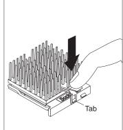
**Note:** Thermal grease is used to seal the heat sink to the microprocessor. Be careful not to get the grease on your skin. If the grease touches your skin or clothing, wash the area with soap and water.
