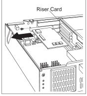
${f 2}$  Remove the adapter and insert it into a static-protective package.
