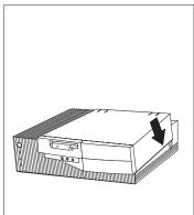
**4** Make sure you can see the volume control knob through the hole in front of the computer, and then push the cover back until it catches and fits the computer snugly. You should hear the cover click into place.
