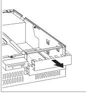
**Note:** If you remove a drive which has removable media from a bay and you do not intend to install a new drive immediately, replace the bay panel and the metal shield.
