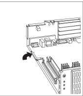
Because you cannot see the connection with the full-sized adapter in place, it is important to engage the system board latch in the support to make sure it is fully seated.
