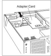
**5** Go to the device-record form in *Using Your Personal Computer*, and write the adapter name next to the slot into which you installed it.
