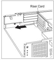
**4** Slide the full-sized adapter into the bottom expansion slot, pressing on both ends to make sure it is properly seated in the riser card.
