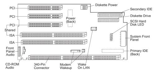
**Note:** The diskette and IDE drive connectors are also on the riser card. When installing optional drives, refer to this illustration.
