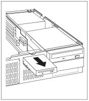
${f 3}$  Disassemble the drive from the bracket outside of the computer, loosening and removing the screws from the sides of the diskette drive bracket.
