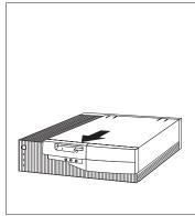
**4** Lift the back edge and slide the cover forward until it comes free.
