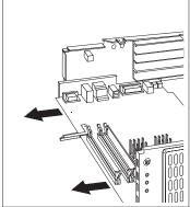
**3** Remove the bottom expansion slot screw and cover.
