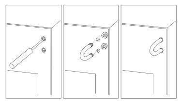
**3** If you cannot access the nuts with the wrench, you will need to remove the side cover. See "Disconnecting Cables and Removing the Cover" on page 6.
