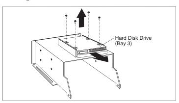
${f 3}$  Place the removed drive in a static-protective package.
