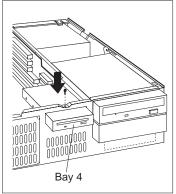
**3** Attach the power and signal cables. Refer to "Adapters and the Riser Card" on page 27 for an illustration showing the locations of the connectors on the riser card.
