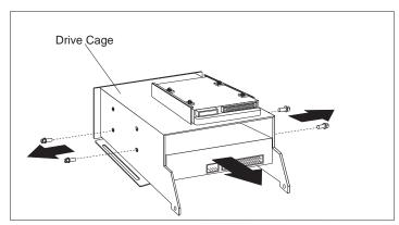
b. To remove a 3.5-inch hard disk drive from bay 3, you must remove the screws from the bottom of the drive, then slide the drive out of the bay. The following illustration shows the screws being removed from the drive and the drive cage.
