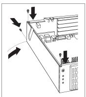
${f 3}$  Align the holes and insert the three screws.
