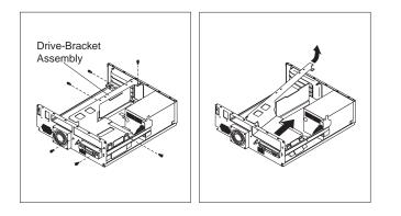
**6** If you want to remove the drive in bay 2, remove the four screws that secure the drive to the drive-bracket assembly.
