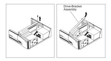
**4** To remove a drive in bay 2 or bay 3, disconnect the cables from any drives in bays 1, 2, and 3.
