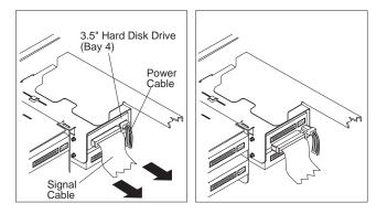
**5** Remove the screw securing the drive-bracket assembly and then remove the assembly from the computer.
