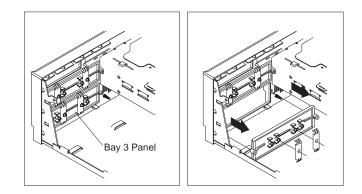
**13** Reinstall the drive-support bracket.
