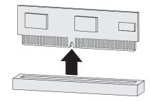
**4** Position the module so that the notch on the bottom edge aligns with the notch in the connector. Insert the bottom edge of the memory module into the connector and push down evenly. Make sure the module is fully inserted into the connector.
