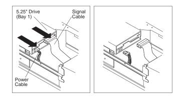
**3** Remove the four screws securing the drive in bay 1, and then remove the drive.
