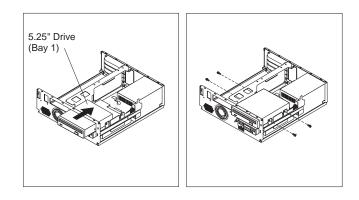
**12** Connect all signal and power cables to the drive in bay 1.
