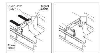
$\mathbf{2}$  Remove the drive in bay 1 from the drive-bracket assembly.
