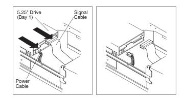
${f 5}$  Remove the drive in bay 1 from the drive-bracket assembly.
