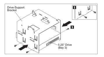
**12** If you installed a drive other than a hard disk drive, remove the bay panel for bay 3.
