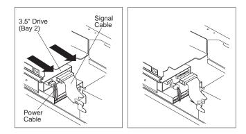
**5** Remove the six screws that secure the drive-bracket assembly, and then remove the assembly from the computer.
