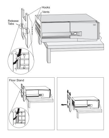
Installing and Removing the Optional Floor Stand
