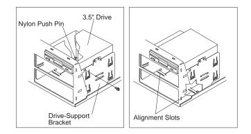
**8** Slide the bracket slightly to the rear, then up and out of the computer.
