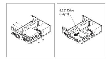
**3** Disconnect the signal and power cables from the installed drives in bays 2 and 3.
