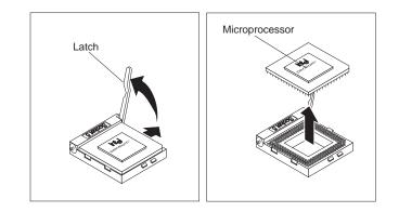
**7** Store the old microprocessor in a static-protective package. Make a note of the microprocessor type for future reference.
