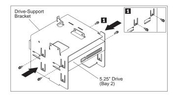
**10** If you installed a drive other than a hard disk drive, remove the bay panel for bay 2.
