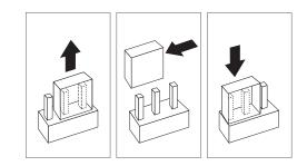
**4** Wait one minute and then move the jumper back to its normal position (pins 2 and 3). You are now able to set a new password.
