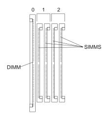
**1** Note the slot position of any adapters that block access to the DIMM connector, and then remove these adapters. (In most cases, it is not necessary to remove half-length adapters.) For information about removing an adapter, see page 12.
