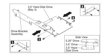
**9** Reinstall the drive-bracket assembly in the computer.
