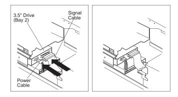
**10** Reinstall the drive in bay 1 of the drive-bracket assembly. Align the screw holes in the side of the drive with the front set of screw holes in the drive-bracket assembly.
