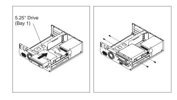
**16** Reconnect the signal and power cables to the drive in bay 1.
