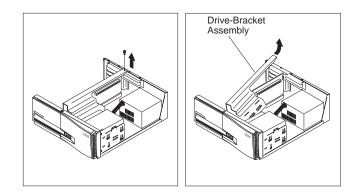
**6** To install a drive in bay 2 or bay 3, disconnect the cables from the drives in bays 1, 2, and 3.
