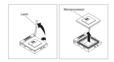
**10** Touch the static-protective package to any *unpainted* metal surface on the computer; then remove the microprocessor from the static-protective package.
