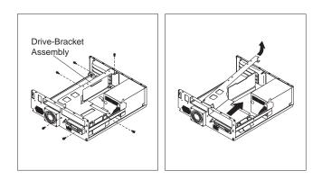
**8** Install the drive into bay 3 of the drive-bracket assembly.
