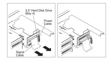
**3** Remove the screw securing the drive-bracket assembly, then remove the assembly from the computer.
