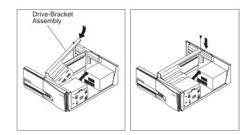
**18** Connect the signal and power cables to each of the installed drives. Connecting cables to the drive in bay 4 is shown to illustrate this procedure.
