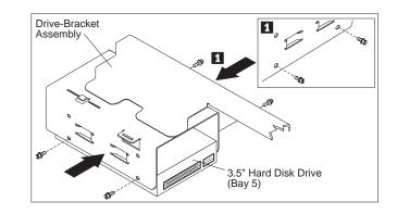
17 Reinstall the drive-bracket assembly and secure it with the screw.
