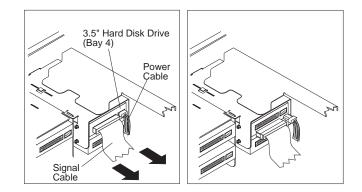
$\mathbf{2}$  Remove the drive-bracket assembly from the computer.
