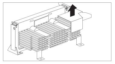
**2** Remove the two screws holding the bottom bracket to the system board, then pull the bracket forward and lift it out, as shown in the following diagram.
