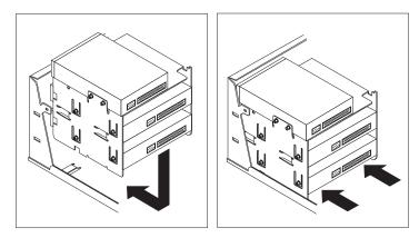
${f 3}$  Insert and tighten the screw of the drive-support bracket to the computer frame.
