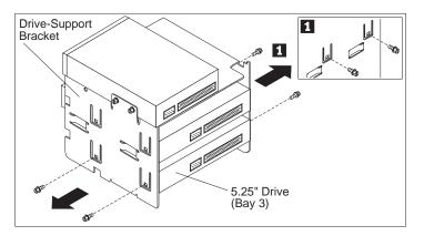
b. If you have installed a 3.5-inch hard disk drive, a mounting bracket holds the drive in place. The following illustration shows the mounting bracket being removed from the drive-support bracket.
