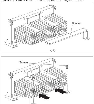
${\bf 5}~$  Insert the two screws in the bracket and tighten them.
