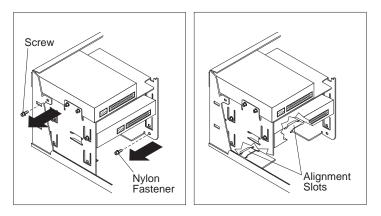
${\bf 3}$  Gently slide the bracket backwards to clear the alignment slots, and then lift the bracket out of the computer.
