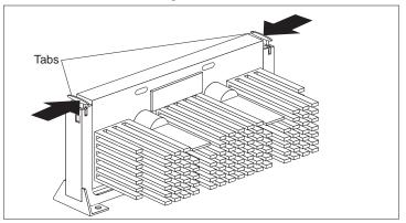
**4** Carefully place one hand on the system board and pull the microprocessor up and out of the connector with the other hand.
