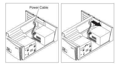
**3** Remove the stabilizer clip and the drive-bracket assembly. For instructions, see "Removing the Drive-Bracket Assembly" on page 14.
