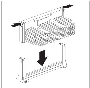
**4** Slide the bottom bracket over the bottom row of heat sink tines, aligning the screw-holes on the bracket with the holes on the system board.
