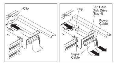
**3** Clear any cables that might impede the replacement of the cover.
