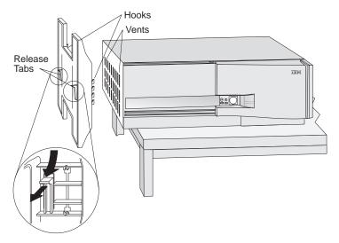
**4** Slide the stand downward and remove it from the computer cover. Be sure to hold onto the floor stand to prevent it from falling after it is released from the cover.
