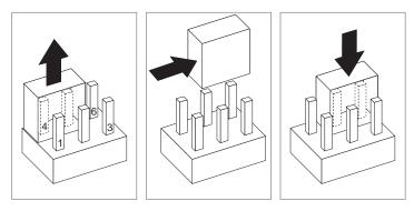
**4** To allow read-only diskette operation, move the jumper from its normal position (pins 5 and 6) to pins 4 and 5.
