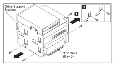
c. You can then remove the hard disk drive from the mounting bracket, as shown in one of the following illustrations.
