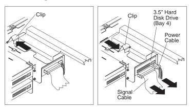
**3** At the rear of the computer, remove the screw and lift the drive-bracket assembly from the frame of the computer.
