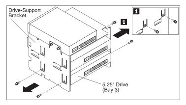
b. If your computer comes with a 3.5-inch SCSI hard disk drive installed in bay 3, a mounting bracket holds the drive in place. The following illustration shows the mounting bracket being removed from the drive-support bracket.
