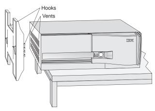
**4** Hold the floor stand firmly against the computer and slide the stand upward. You will feel the floor stand snap into place. Check the stand to make sure it is securely attached.
