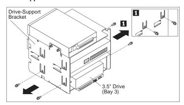
c. You can remove the SCSI hard disk drive from the mounting bracket. The following illustration shows the drive being removed from the mounting bracket.
