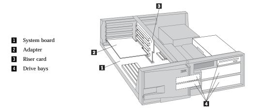
Your computer comes with a graphics adapter installed on the riser card, a diskette drive installed in a drive bay, and a hard disk drive installed in a drive bay.
