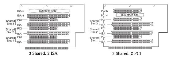
**Note:** Except for adapters installed on the single-slot side, adapters plug into the PCI slots with the components facing down and adapters plug into the ISA slots with the components facing up.
