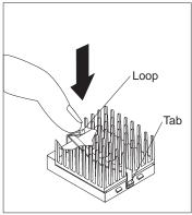
**Note:** A thermal grease is used to seal the heat sink to the microprocessor. If the heat sink is permanently cemented to the microprocessor, you can remove both the heat sink and the microprocessor after you lift the lever in step 3. Also, be careful not to get the grease on your skin. If the grease touches your skin, wash the area with soap and water.
