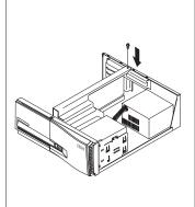
**3** Reconnect the cables to any drives that are housed in the drive-bracket assembly. The following illustrations show power and signal cables being connected to a drive in bay 4.
