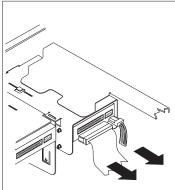
${f 2}$  At the rear of the computer, remove the screw and lift the drive-bracket assembly from the frame of the computer.
