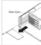
**3** If you are not installing another adapter in this slot, install an expansion-slot cover. The following illustrations show the expansion-slot cover being installed.
