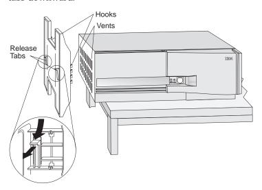
**4** Slide the stand downward and remove it from the computer cover. Be sure to hold onto the floor stand to prevent it from falling after it is released from the cover.
