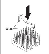
$oldsymbol{8}$  Press down on the loop to rehook the clip to the tabs on the connector.
