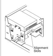
${f 3}$  Gently slide the bracket backwards to clear the alignment slots, and then lift the bracket out of the computer.
