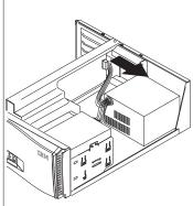
${f 3}$  Remove the drive-bracket assembly. For instructions, see "Removing the Drive-Bracket Assembly" on page 14.
