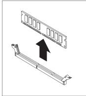
**3** Store the DIMM in a static-protective package.
