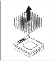
**3** Release the lever on the side of the microprocessor connector and lift it all the way up. This releases the microprocessor. Lift the microprocessor out of the socket.
