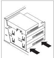
${f 3}$  Insert and tighten the screw of the drive-support bracket to the computer frame.
