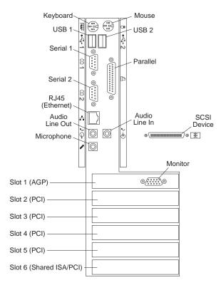
Figure 2. Rear Connector Panel and Expansion Slots
