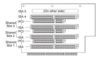
Figure 1. Riser Card for the PC 300XL and IntelliStation M Pro
