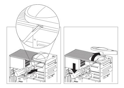
**c** Remove the top-handle screw and the screw from the drive support bracket. Next, move the drive cage towards the power supply until it stops, and then lift it away from the computer.
