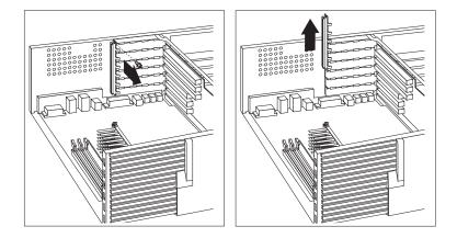
**2** Remove the appropriate expansion-slot cover.
