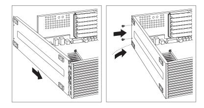
${f 3}$  Align the holes and insert the two screws.
