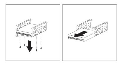
If your drive is installed with side screws and grommets, as shown in the second illustration, leave the grommets in the holes when removing the drive. The following illustration shows a drive removed this way.
