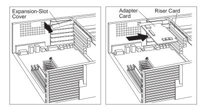
**3** Install the bracket and the screw.
