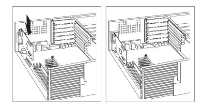
**Note:** Some adapters support the attachment of *daughter cards*. Because a daughter card might provide another connector for external devices, a second slot is provided on the computer wall for access.
