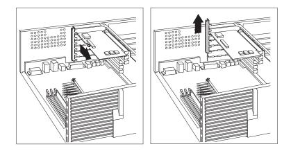
**2** Disconnect any cables attached to the adapter, remove it, and insert it into a static-protective package. If you are not installing another adapter in this slot, install an expansion-slot cover.
