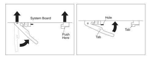
**Note:** You cannot see the connection with a full-sized adapter in place. To make sure the system board is fully seated, it is important that the tab on the right-hand rail is engaged in the opening in the chassis.
