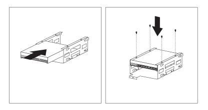
To install a drive that uses side screws and grommets for installation, insert the grommet into the large part of the hole (if not already installed), as demonstrated below, and slide it into the smaller part of the hole. Once the grommet is installed, slide the drive into the bay and tighten the screws in the hole.
