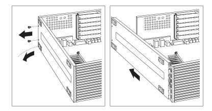
${\bf 2}$  Slide the tabs on the end of the cover out of their openings and remove the cover.
