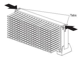
**3** Carefully place one hand on the computer frame and with the other hand pull the microprocessor up and out of the connector.
