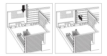
**Note:** Removing an adapter frees up system resources. If you remove an ISA legacy adapter, you must use the Configuration/Setup Utility program to set the previously used resources to [**Available**]. For more information, see Chapter 7, "Completing the Installation" on page 66.
