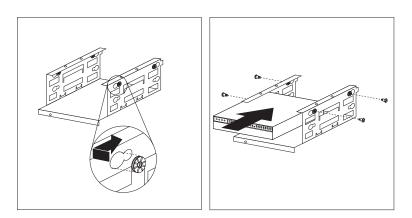
• To remove a drive, remove the screws holding the drive in the cage and slide the drive out of the cage.
