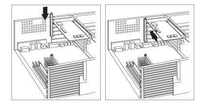
**4** If you installed a network adapter that uses Wake on LAN or Alert on LAN, attach the cable from the riser card to the adapter. See page 22 to locate the Wake on LAN or Alert on LAN connectors. If you installed a modem and want to use Modem Wakeup, see page 22 to locate the Modem Wakeup connector on the riser card.
