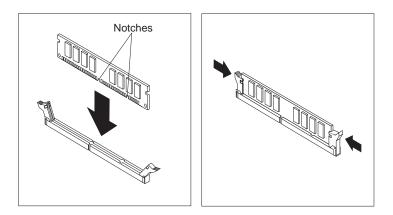
**5** Firmly push the module straight down into the connector until the retaining clips pop up and snugly fit around both ends of the module.
