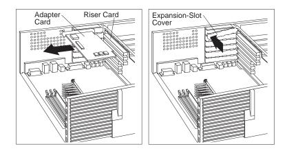
${f 3}$  Install the bracket and the screw.
