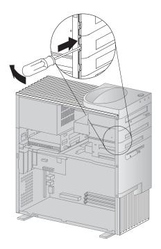
${f 3}$  Remove the two screws holding the drive and slide it out the front of the computer.
