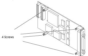
5. Position the selectable PMC card over the base adapter with the component sides of both the selectable PMC card and the base adapter facing each other.
