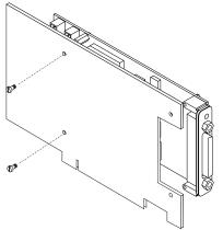
7. Taking care not to damage the rubber gasket around the connector on the selectable PMC card, align the adapter bracket as shown and install the remaining two screws.
