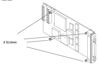
2. Align the connector on the PMC card with the connector on the base adapter.
