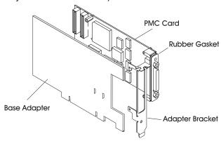
9. Carefully separate the connector on the PMC card from the connector on the base adapter using a gentle rocking motion.
