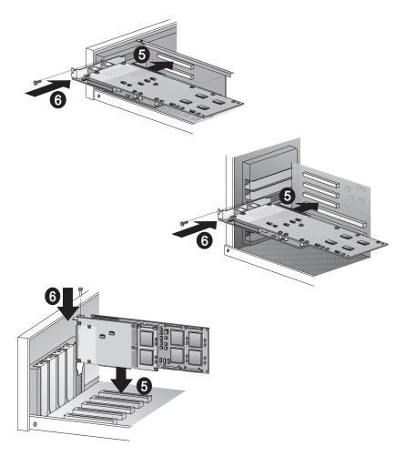
Figure 2-4. Inserting the Adapter
