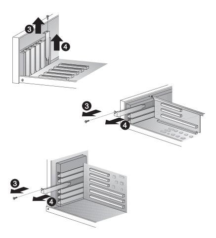
Figure 2-3. Removing the Expansion Plate
