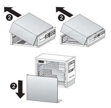
Figure 2-2. Removing the Computer Cover
