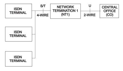
Figure 1-3. ISDN Reference Model for BRI S/T and U
