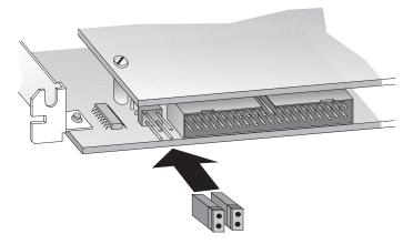
Figure 2-5. Electrically Terminating the MVIP Bus
