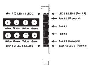
Figure 8-1. Adapter LED Arrangement
