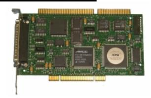
ARTIC is an acronym for A Realtime Interface Coprocessor. The ARTIC family of general-purpose coprocessor adapters can off-load realtime demands, facilitate high-speed communication tasks, and provide front-end processing for a variety of communications data.
