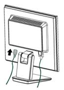
5. Insert the power plug into a properly grounded electrical outlet.
