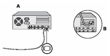
4. Attach the power cord at the back of the monitor where it says "AC IN". The arrow in the drawing below indicates the approximate area:
