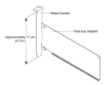
The option package also contains a low-profile expansion-slot bracket that is approximately 7 cm (2.9 in.) long. If the opening for the PCI-X or PCIe expansion slot is approximately 6 cm (2.3 in.) long, you must replace the preinstalled bracket with the low-profile bracket. You will do this in step 6 on page 15 in the following procedure.
