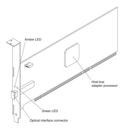
The major components of the dual-port host bus adapter (PCI-X or PCI Express) are shown in the following illustration.
