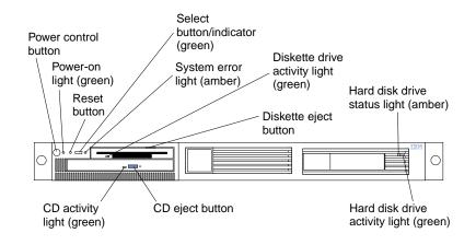
Power-control button: Press this button to manually turn the server on or off.
