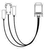
**Keyboard connector:** There is one keyboard connector on the end of the device breakout cable. This connector is identified by the keyboard icon.
