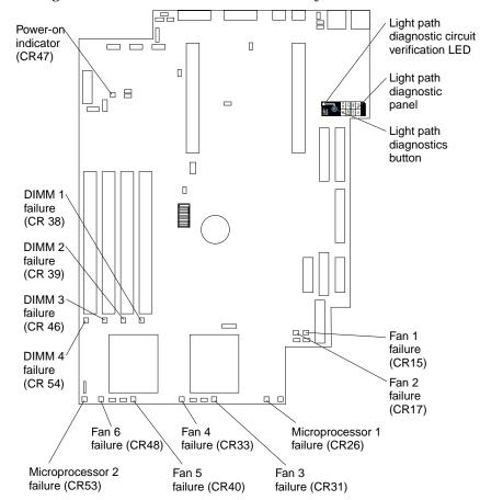
The following illustration identifies the LEDs on the system board.
