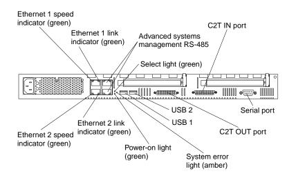
**Ethernet 1 speed indicator:** This green LED lights when the speed of the Ethernet LAN that is connected to Ethernet port 1 is 100 Mbps.
