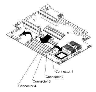
c. When installing a memory module be sure that no gap exists between the DIMM and the retaining clips. If a gap does exist between the memory module and the retaining clips: open the retaining clips, remove the DIMM; then, reinsert the DIMM properly.
