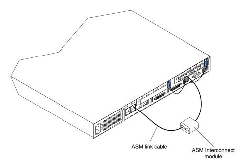
2. Connect one end of the ASM link cable (Cat 5 or 3 Ethernet cable) to the RS- 485 port.
