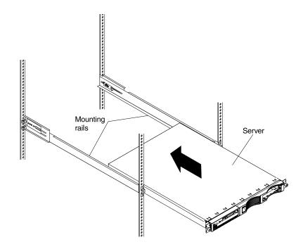
3. Using the thumb screws on the front of the server; secure the server to the brackets.
