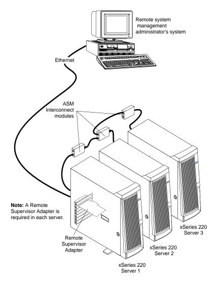
**Note:** The ASM Interconnect module is attached to the RS-485 P-P (peer to peer) port on the back panel of the Remote Supervisor Adapter in each server.
