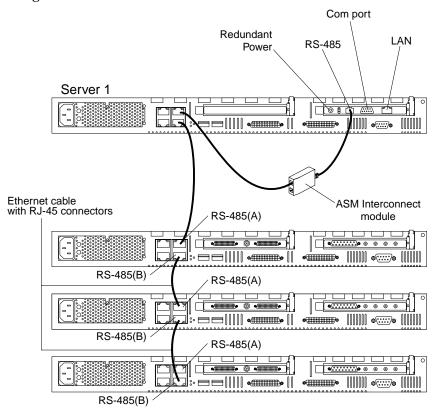
In the following example, an Ethernet cable is connected to the Remote Supervisor Adapter that is installed in an xSeries 220. In this case, the xSeries 220 uses the LAN connection to forward system-management data generated by the other servers in the ASM interconnect network bus to the remote system-management administrator.
