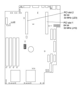
To install the Remote Supervisor Adapter, complete the following steps:
