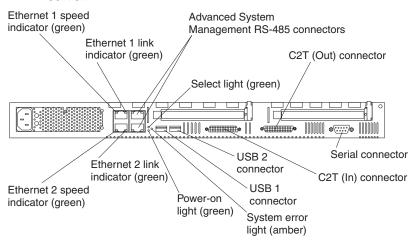
The ASM connectors on the back of the server are referred to in this book as RS-485 (A) and RS-485 (B).
