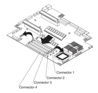
When installing a memory module be sure that no gap exists between the DIMM and the retaining clips. If a gap does exist between the memory module and the retaining clips: open the retaining clips, remove the DIMM; then, reinsert the DIMM properly.
