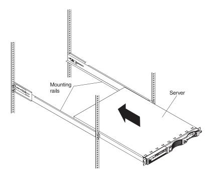
3. Using the thumb screws on the front of the server/workstation; secure the server/workstation to the brackets.
