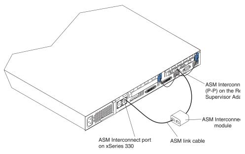
2. Connect one end of the ASM link cable (Cat 5 or 3 Ethernet cable) to the ASM Interconnect module, and connect the other end of the link cable to the RS-485 port.
