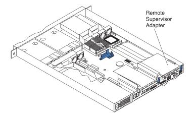
7. Connect the internal cables to the adapter. Note that the 20-pin ribbon cable (see "Inventory checklist" on page 60), which connects the system management connector on the Remote Supervisor Adapter to the system board at J57 (see "System board options connectors" on page 44), also supplies power to the adapter.
