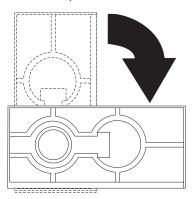
When you are finished and have reinstalled the side cover, turn the two front stabilizing feet a quarter turn outward and set the computer carefully back on its feet.
