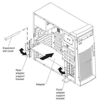
**Attention:** Be certain that the adapter is correctly seated in the expansion slot before you turn on the computer. Incomplete installation of an adapter might damage the system board or the adapter.
