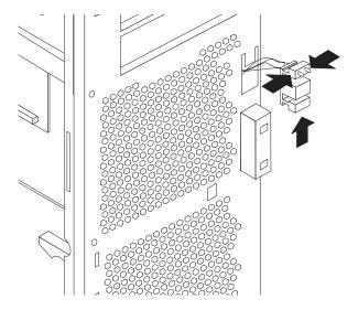
5. Disengage the lower tab of the power/LED switch by pressing upward on the lower tab of the power/LED switch until it comes loose.
