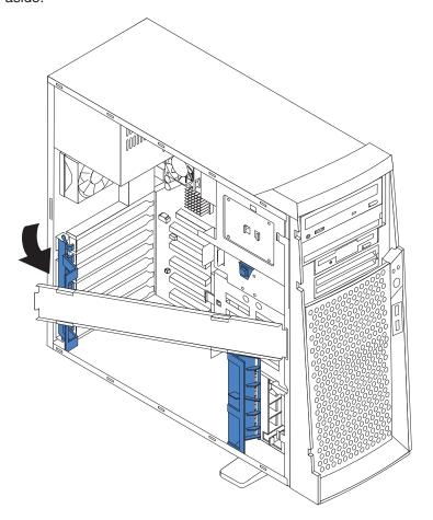
To reinstall the support bracket, reverse the previous steps.
