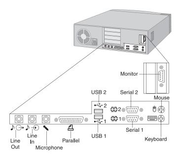
**Note:** The connectors on the rear of the computer have color-coded icons. You can use the icons to determine where to connect cables on your computer.
