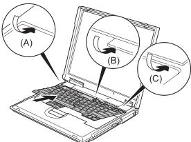
Push the Y key 1 to connect the keyboard to the connector on the underside of the key; then push the frame of the keyboard 2 to latch the latches.
