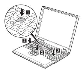
After the fastening of two screws of bottom side, push the Y key again to connect the keyboard firmly to the connector on the underside of the key.
