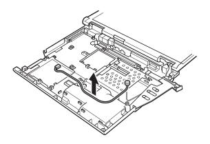
**Cable routing:** When replacing the cable, see the following figure for its routing.
