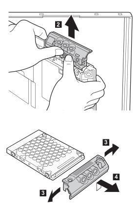
When installing: Make sure that the HDD connector is firmly connected.
