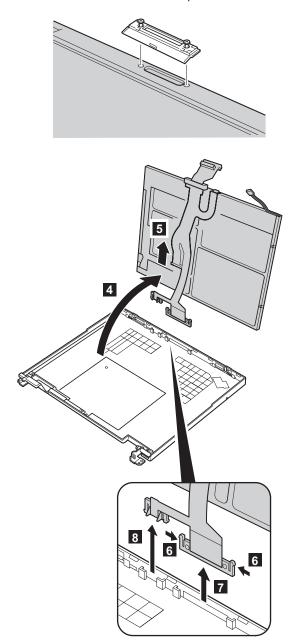
Cable routing: When installing the LCD, see the following figure for the routing of the connector cable.
