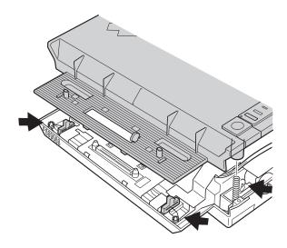
The device release lever is seated correctly.
