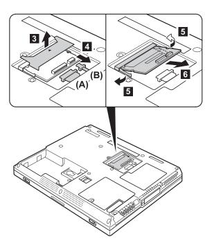
When installing: Make sure not to pinch the connector cable when re-installing the Mini PCI adapter.
