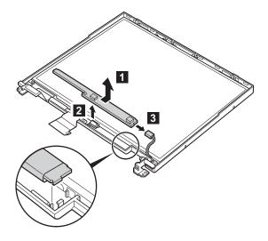
**Cable routing:** When replacing the inverter card, see the following figure for the routing of the connector cable.
