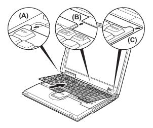
Push the Y key 1 to connect the keyboard to the connector on the underside of the key; then push the frame of the keyboard 2 to latch the latches.
