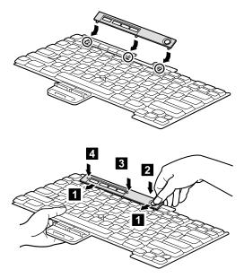
When installing: When installing the keyboard, do as follows:
