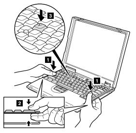
To make sure that the front side of the keyboard is housed firmly, gently press the Shift keys with your
