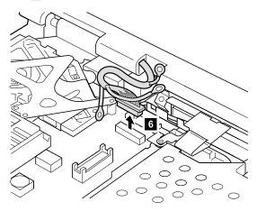
When installing: Make sure that the LCD cable connector is firmly attached and then tighten the screws of each terminals.
