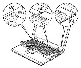
Insert your fingers into the PC Card slot on the left of the computer and the Ultrabay 2000 slot on the right of the computer as shown in 1. Then, with your fingers in those slots as in 2, latch the keyboard in place by using your thumbs to press firmly on the Shift keys. Press the Y key to connect the keyboard to the connector on the under side of the key 3.
