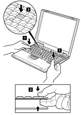
3. To make sure that the front side of the keyboard is housed firmly, gently press the shift keys with your thumbs and try to slide the keyboard towards you. Do not push parts (A) and (B) on the keyboard strongly; to do so might cause distortion of the Ultrabay 2000 slot and the PC Card slot.
