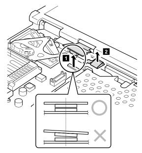
When installing: Make sure that the FPC connector is firmly attached.
