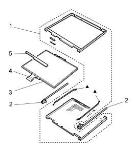
Note: The parts marked with ▲ are only for 13.3-in. LCD cover kit.
