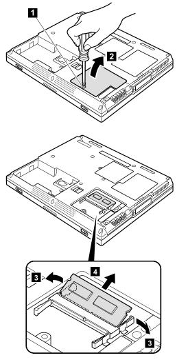
When installing: With the notched end of the DIMM toward the socket, insert the DIMM into the socket, and then press it firmly. Pivot the DIMM until it snaps into place. Make sure that the card is firmly fixed in the slot and does not move easily.
