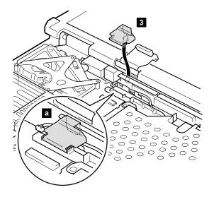
When installing: Make sure that the FPC bracket is firmly attached as shown in the figure a.
