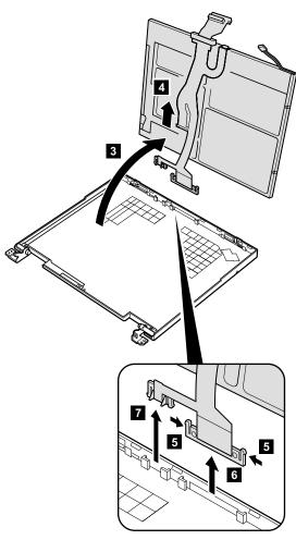
Cable routing: When installing the LCD, route the connector cable as in the following figure:
