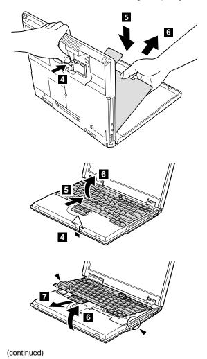
When installing the easy-button cover, do as follows:
