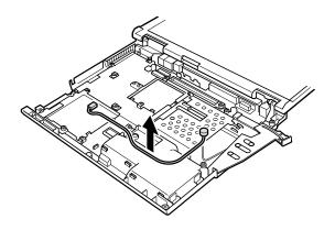
Cable routing: When replacing the cable, make sure the connector is firmly attached into place a. Cable slacking is only allowed at the b -part of the frame.
