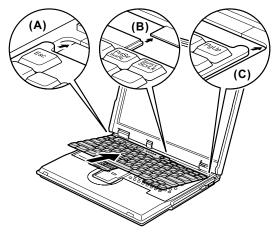
Insert your fingers into the PC Card slot on the left of the computer and the Ultrabay 2000 slot on the right of the computer as shown in 1. Then, with your fingers in those slots as in 2, latch the keyboard in place by using your thumbs to press firmly on the Shift keys. Press the Y key to connect the keyboard to the connector on the under side of the key 3.
