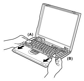
After the fastening of two screws of bottom side, push the Y key again to connect the keyboard firmly to the connector on the underside of the key.
