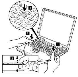
To make sure that the front side of the keyboard is housed firmly, gently press the Shift keys with your thumbs and try to slide the keyboard towards you. Do not push parts (A) and (B) on the keyboard strongly; to do so might cause distortion of the Ultrabay 2000 slot and the PC Card slot.
