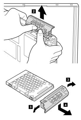
When installing: Make sure that the hard-disk connector is firmly connected.
