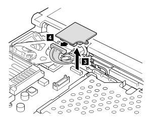
When installing: Make sure that the connectors are firmly attached.
