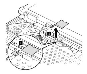
When installing: Make sure that the FPC bracket is firmly attached as shown in the figure a.
