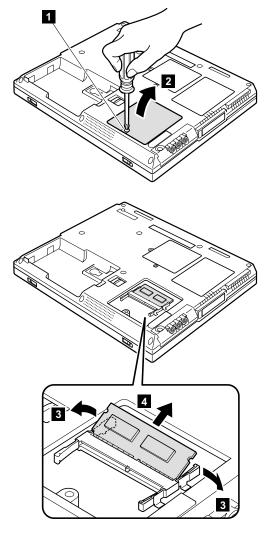
When installing: Make sure that the card is firmly fixed in the slot and cannot be moved easily.
