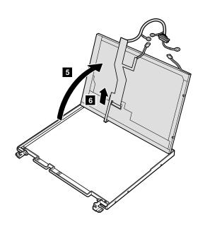
Cable routing: When installing the LCD, route the connector cable as in the following figure:
