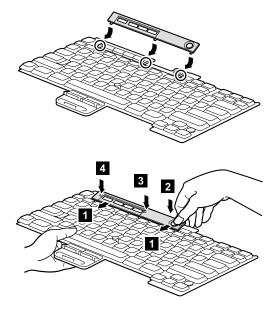
**When installing:** When installing the keyboard, do as follows:
