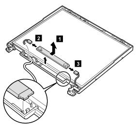
**Cable routing:** When replacing the inverter card, route the connector cable as in the following figure:
