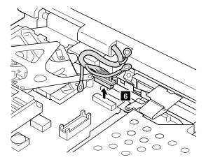
When installing: Make sure that the LCD cable connector is firmly attached and then tighten the screws of each terminals.
